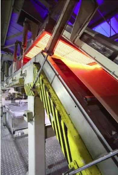
Heraeus Noblelight develops special drying and curing solutions tailored to the production process to optimise the use of energy, reduce costs and save time.
