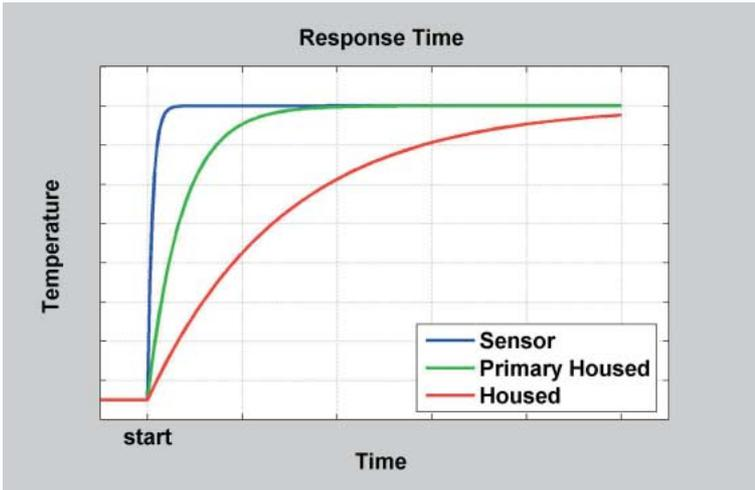
*Figure 3: Short reaction times are very dependent on the type of construction. Joining different materials that are frequently subjected to thermal shocks demands close co-operation in development.*
