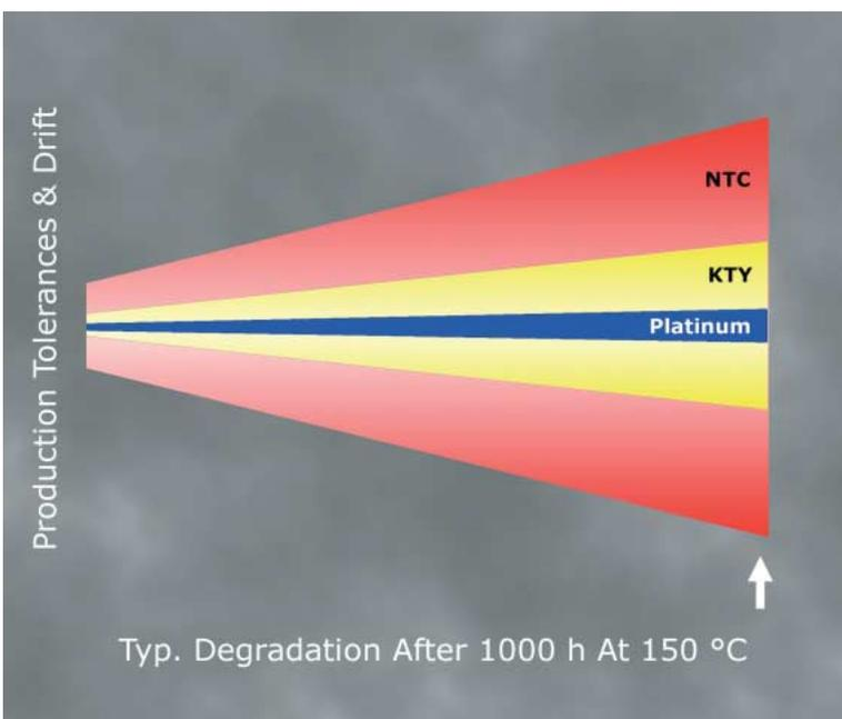
*Figure 2: Typical drift characteristic for different sensor materials. Also from other applications, platinum thin-film technology is well known for its long-term stability.*
