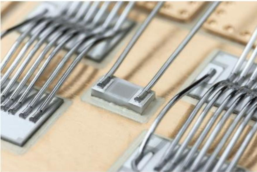
Sinterable temperature sensors for power electronics
