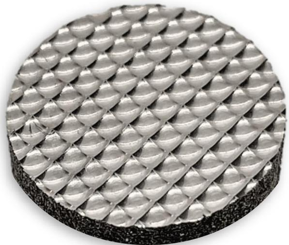
Figure 2: Near-final contour production of highly structured surfaces
