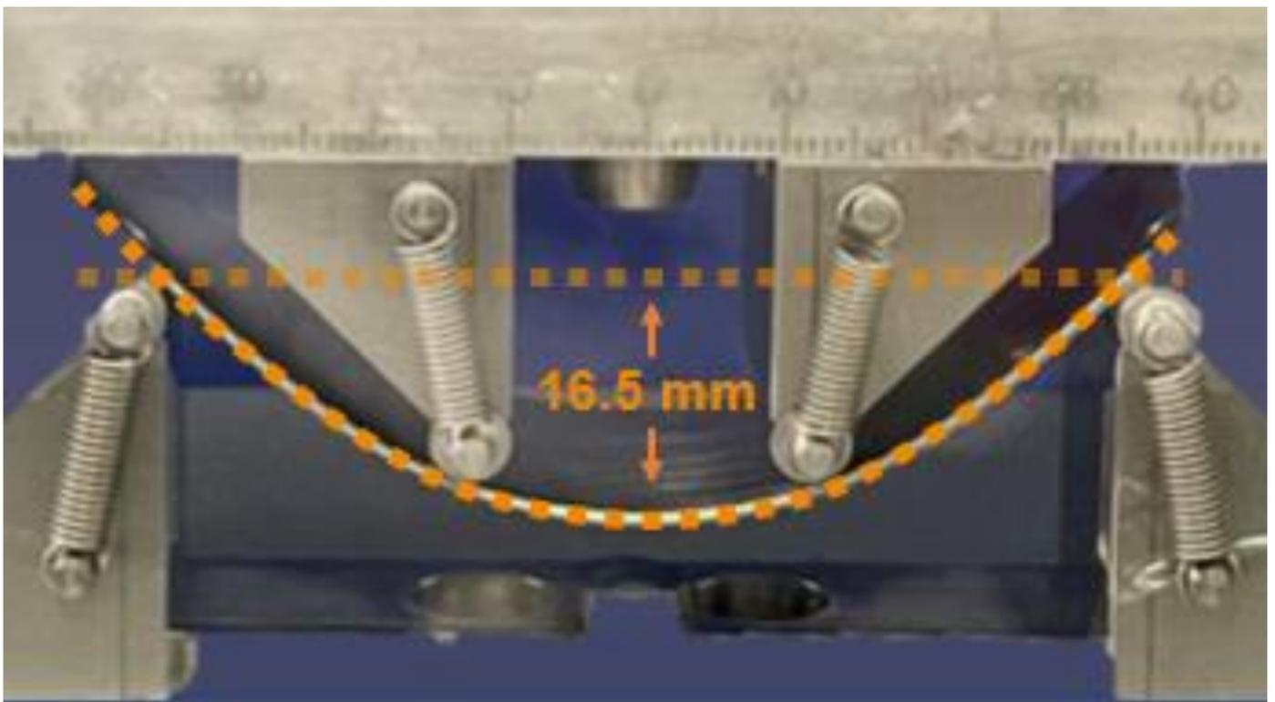
Figure 1: Amorphous plate @ 350 N load, 4-point bending test
