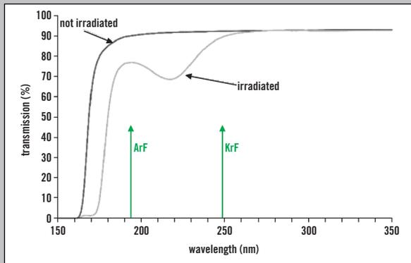
be measured with a photospectrometer in a well defined way. Transmission losses under excimer laser irradiation @ 193 nm and 248 nm are mainly caused by the absorption band at 215 nm (the so called E'-center). Therefore the following statements are valid for both wavelengths.
