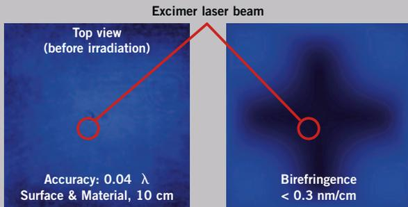
As an example, a cuboid with sides polished to  $0,04 \lambda$  is shown. The sample is illuminated by a circular beam with a homogenous energy density. Because of the irradiation, a compaction/ densification / contraction is observed in the illuminated area. Since the surrounding volume does not contract as much as the irradiated volume, one can observe stress-induced birefringence on the boundary between these regions.
