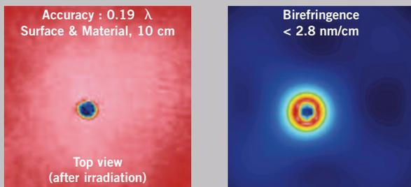
The degree of densification depends upon the irradiation parameters and on the material. In this example, a stress-induced birefringence of  $\sim 3 \text{ nm/cm}$  and a material inhomogeneity (difference in optical path length) of  $0,15 \lambda$  was generated in Suprasil® ArF/KrF. Thus, this example demonstrates very well the need to take radiation-induced effects into consideration in the design of an optical element that is exposed to excimer laser radiation.
