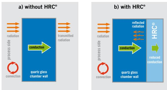
Figure 1: Illustration of the three heat transfer mechanisms.
