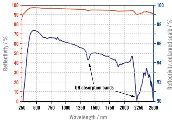
Figure 3: Reflection behavior of a typical HRC® surface.
