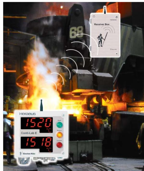
Conti-Lab E instrument variant with radio data transmission
