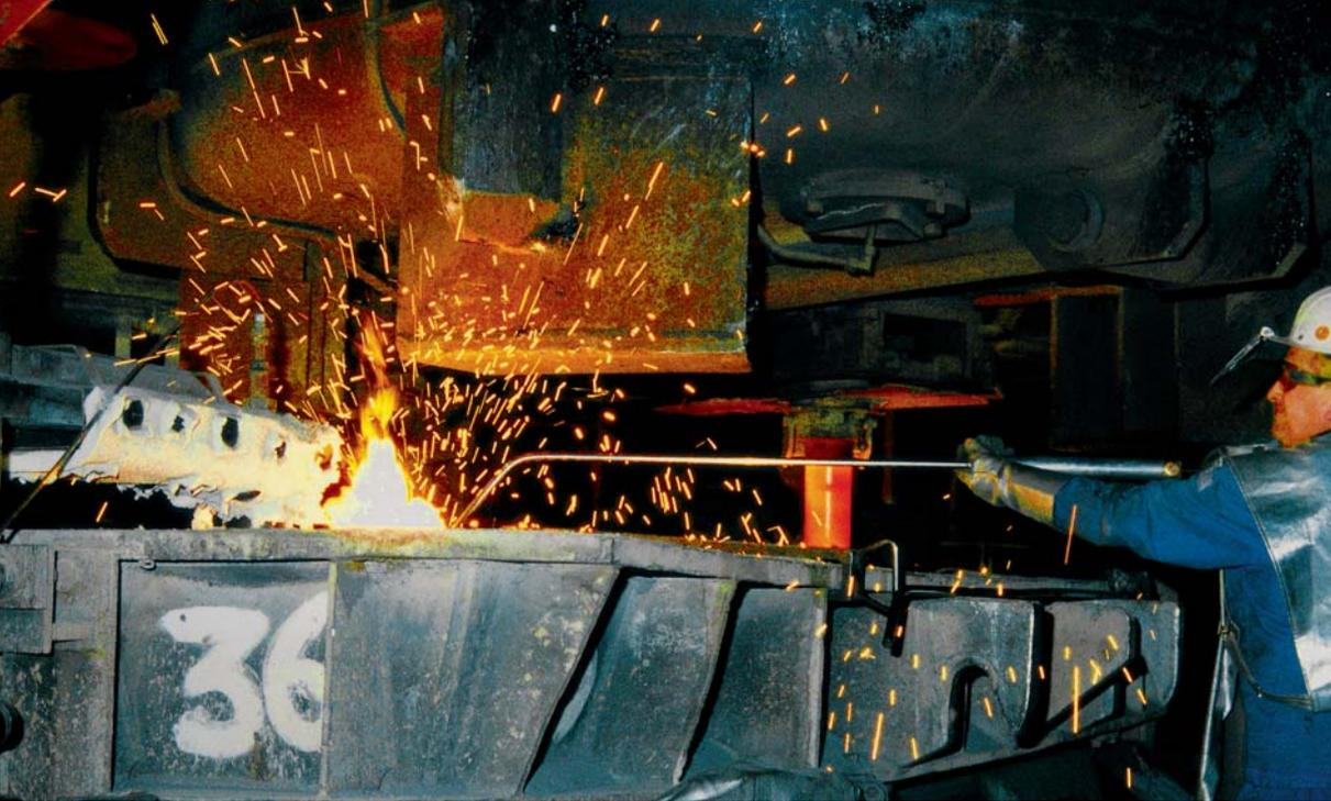
Bath temperature measurement in the tundish
