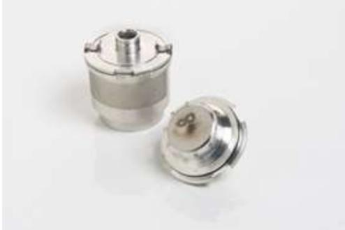
This new design allows its most innovative feature: the preparation-free surface. Moreover, the sample surface is below 200°C when it is removed from the Multi-Lance, ensuring a correct analysis using the QuiK-Lab.
