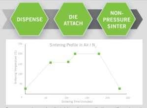
$\label{process_parameters} \mbox{Process parameters can be adjusted depending on application specific requirements}$
