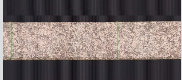
Fine grained and homogeneous texture of Cu ribbons
