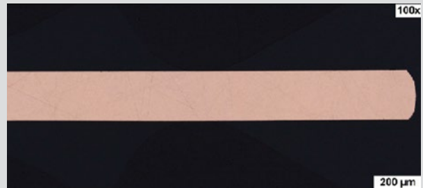
Cross section of PowerCu Soft ribbon with natural rounded and burr-free edge
