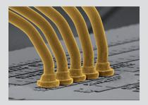
This wire type contains other doping elements apart from the well established beryllium. Due to this doping, type HD3 has a higher strength, loop stiffness and thermal stability than type HD2. Loop stability can also be guaranteed with thinner wire diameters and in flatter and/or long loops.
