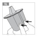
Compress the mould between your hands (at the bottom of the green part) to release the spacer from the surfaces. A cracking sound indicates that it has detached.
