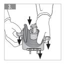
When the cement has completely cured\*, remove or break off the sliding clips.
