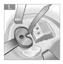
Completely remove the infected prosthesis and residual cement.
