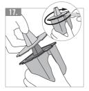
Loosen the tibia cap all around with the help of a flat instrument to remove it afterwards.
