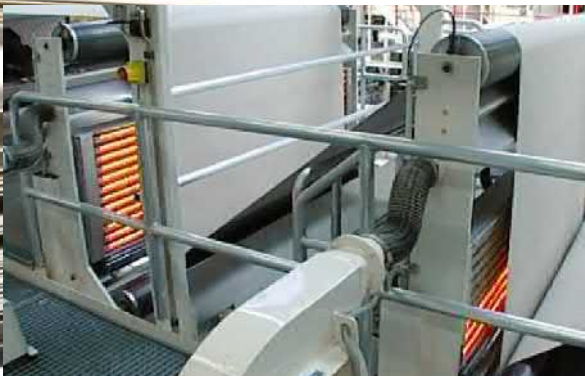
Flexoprinting with Carbon emitters
