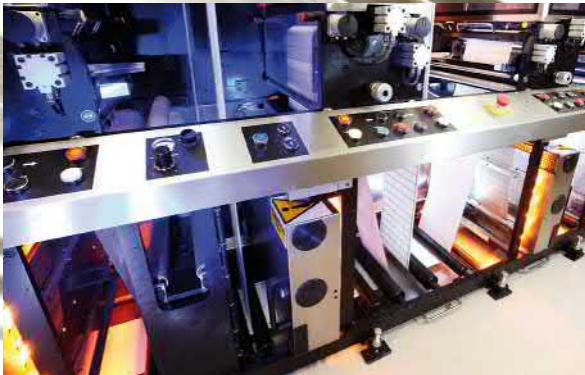
In-line drying of flexo print
