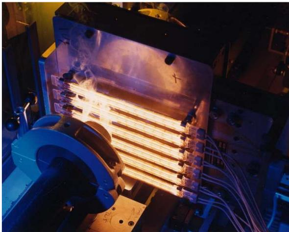
Infrared emitters are arranged in movable plattens that they can be positioned between two pipes. During a few seconds the pipe ends can be welded together.
