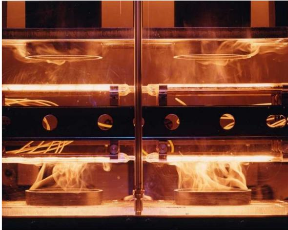
Cylindrical water containers are made of two halves that are welded together afterwards. Tests have shown that the connection is impermeable to liquid and can withstand high pressure.
