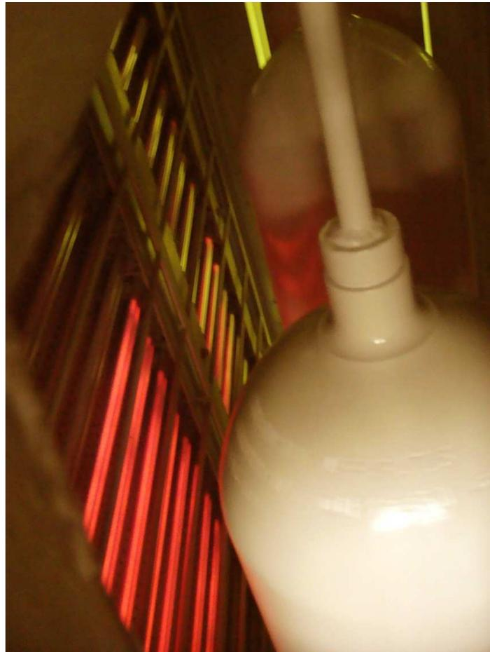
in only a few seconds. The IR drying station is featured with medium wave emitters. Due to a suitable emitter position, the IR drying station can be adjusted to different bottle thicknesses. As a result of the compact system the coating station could be retrofitted in the production line by saving space. Furthermore the emitters react almost instantaneously, that makes it possible to shut them off even during operating stops that saves energy and costs.
