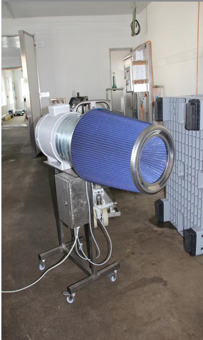
Ozone-free lamps with 254nm UV emission, control unit with 200 W energy consumption and precisely fitting clamping springs.
