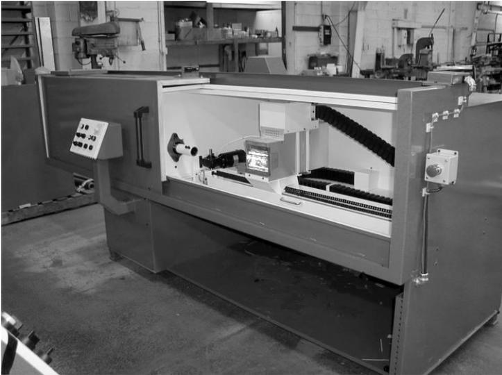
The photo shown at left is a gel coat UV curing station built for curing a clear gel coat onto SCBA tank cylinders used by fire fighters, scuba divers, etc. After application of the gel coat, the cylinder is placed into the unit and one microwave-powered UV lamp traverses the length of the part while the part spins.
