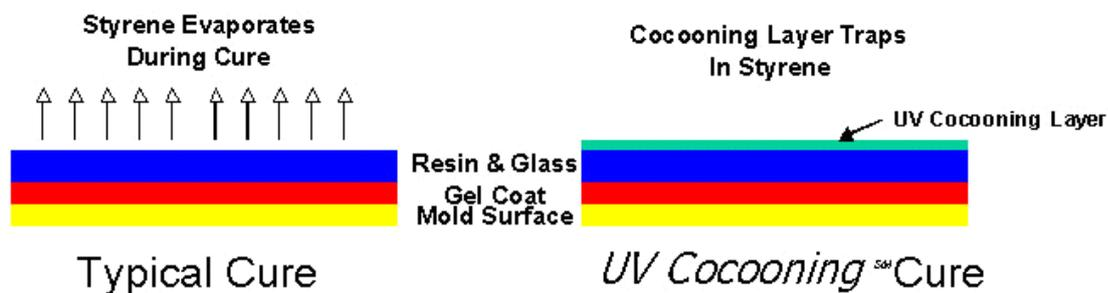
Initial testing using high-powered UV lamps to scan over a part surface, called "UV cocooning" indicates that as much as 40% of styrene emissions may be eliminated. The shape of the part, the amount of photoinitiator used, the number of UV lamps and orientation to the part, and type of resin all impact the emission reduction possible. Of course this also reduces the styrene smell in the workspace and surrounding community. So employee retention may improve and community complaints may decrease.
