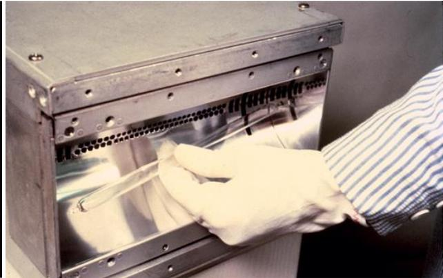
UV LED curing systems, commercial since the mid 2000's, use light emitting diode technology to emit essentially monochromatic UV energy at 365, 385, 395 or 405 nm wavelengths. Individual LEDs are packed into arrays behind an emission window of a UV LED curing system. For efficient operation and long life the LEDs must be cooled, but it's significantly less compared to traditional technologies and often self-contained inside the small form factor and light weight lamp heads.
