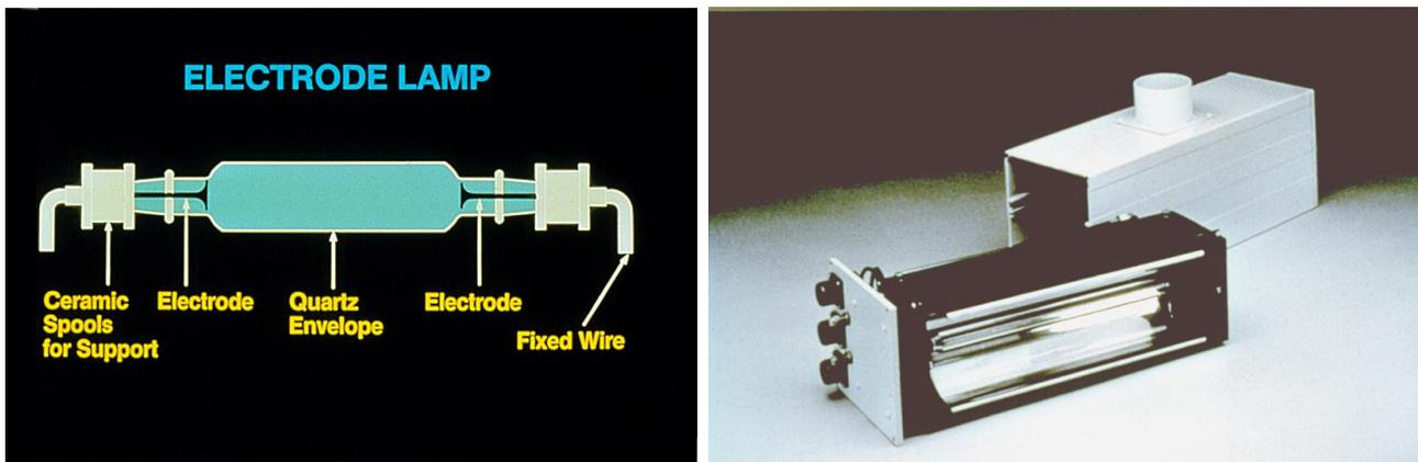
Microwave-powered lamps (also referred to as electrodeless type) are simply a totally enclosed quartz tube. Instead of striking an arc between two electrodes to excite the gasses in the bulb, microwave energy penetrates the quartz to excite the gasses.
