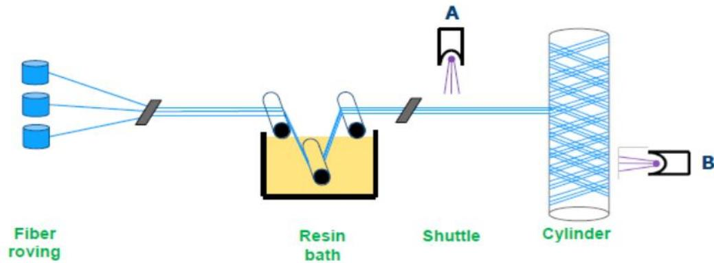
UV lamps can often be retrofitted to existing filament winding machines. For B-stage curing, traditional UV or UV LED lamps are placed above and/or below the rovings, either glass, aramid or carbon, immediately after the resin bath (position A shown above).
