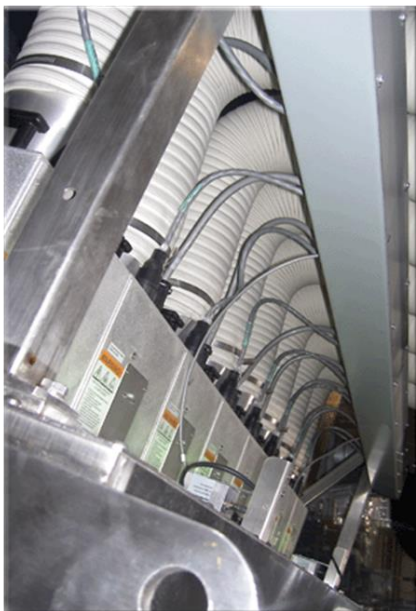
Erickson cures the scratch resistant hardcoat with a bank of Fusion VPS6/1600 lamps.
