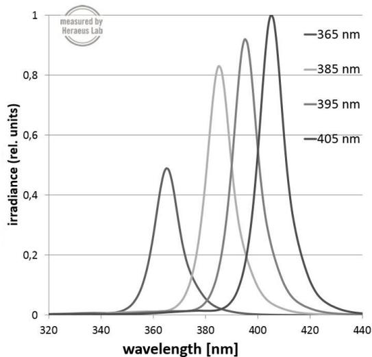
Unlike traditional UV curing which has a broad spectrum output, the output of UV LEDs for curing is currently available in one of three narrow, nearly monochromatic, wavelengths – 365, 385, 395 and 405 nm.
