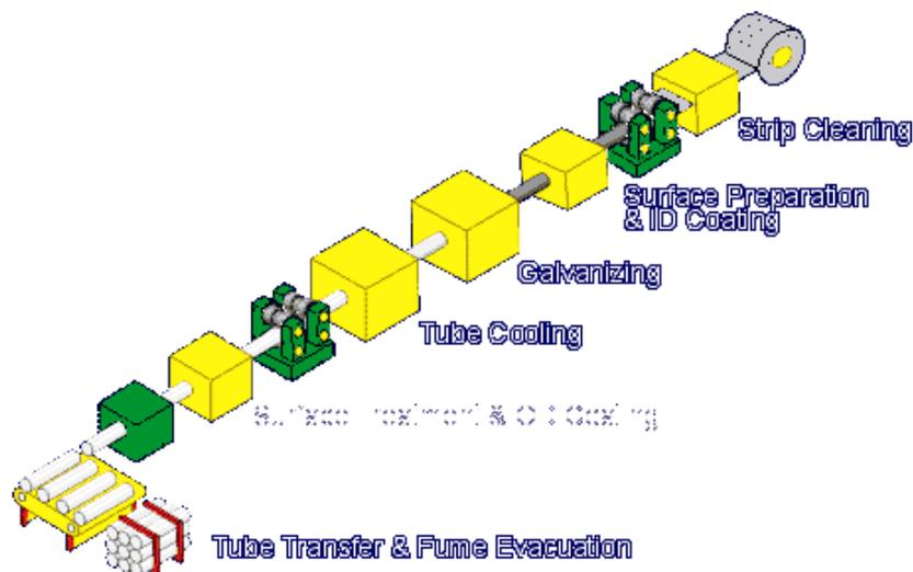
speed from 130 to 250 m/minute) utilizing an increase in line length of only approximately 1.8 meters. The net result of this speed increase with alternative process technologies could be tens of meters.
