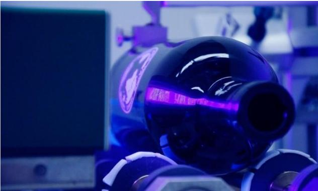
Most glass decorating machine builders offer a UV curing version. These machines can decorate bottles at high speed (150 bottles/min) with excellent color-to-color registration of the printed images. The UV curing capable decorating machines save space because of the elimination of the Lehr. In addition, production can commence any time of the day without having to preheat for an hour or unload the oven, as is the case with a Lehr, saving
