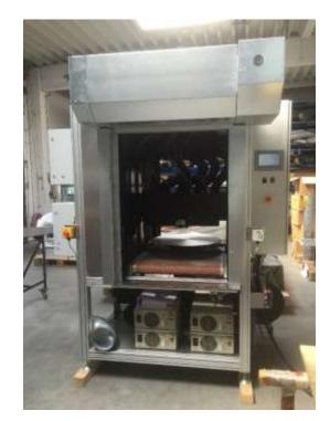
Pilot for post curing of UV 3D printed, additive manufactured parts. Can also cure UV coatings on the completed part.
