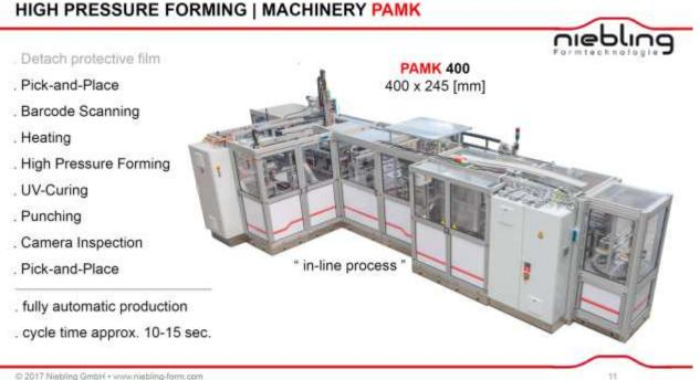
Example of a highly integrated high pressure forming and inmold decorating machine for a turnkey process solution.
