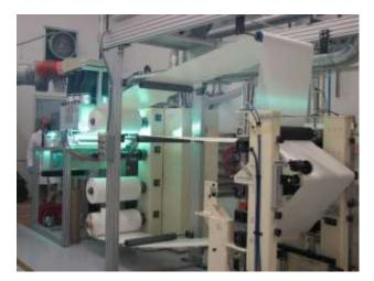
UV curing is used extensively in many graphics arts printing applications such as labels -- for the printing inks, adhesives and the release coatings on the release liner, and for slip resistant coatings on pet food bags,inks and overprint varnishes on food packaging, coatings on engineered functional films, and for ink jet digital printing to name a few.
