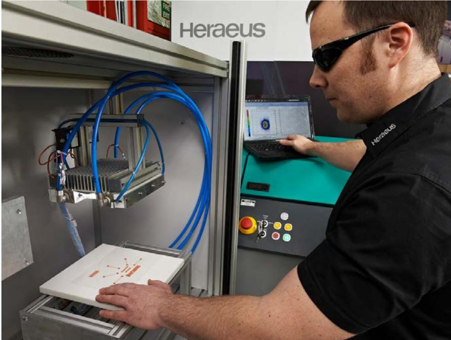
*Setting up a substrate for Photonic exposure.*
