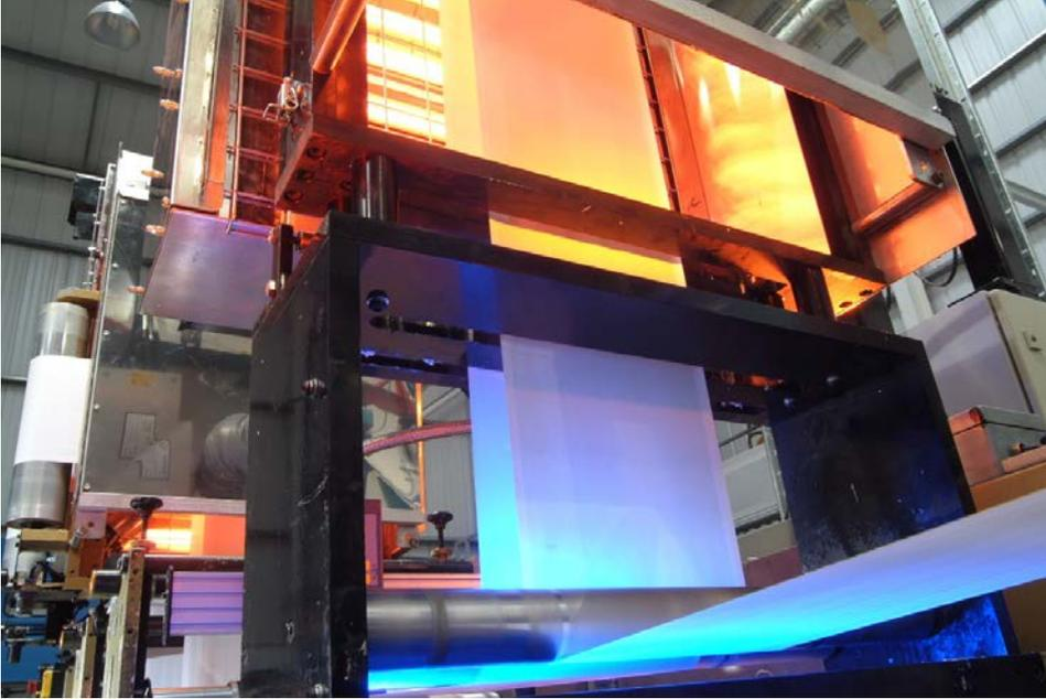
UV radiation cures, infrared heat dries – tests in Application Competence Centers help find the parameters for this.
