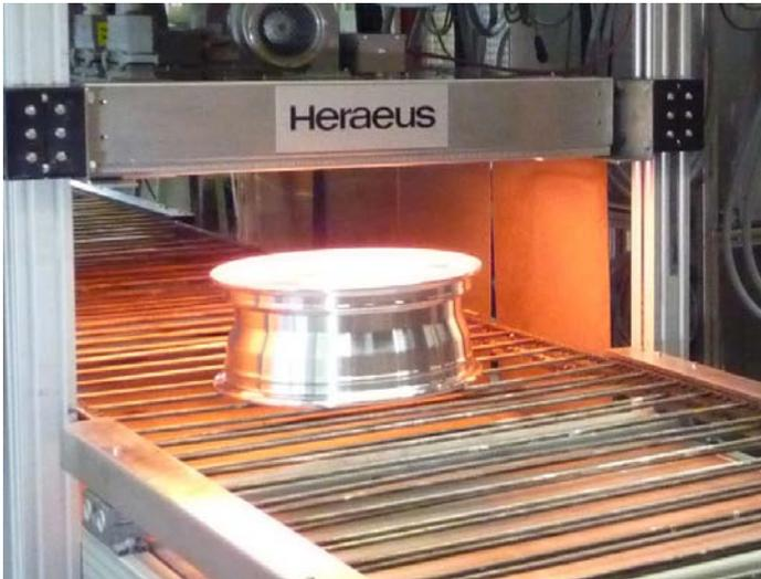
Carbon infrared emitters accelerate the powder coating of aluminium wheels
