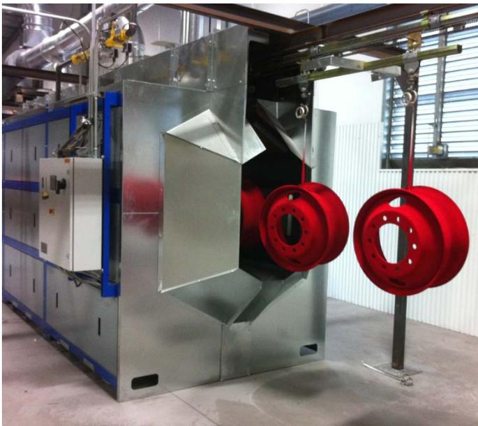
A gas catalytic oven for the gelling and curing of powder coatings
