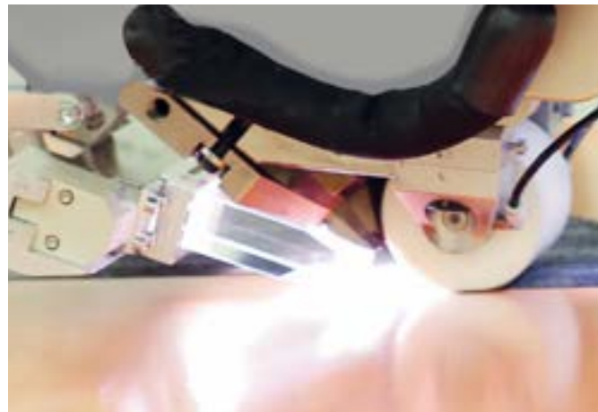
Image 2: a close-up image of the technology laying up the first ply of a dry fibre panel. humm3 ® end effector at Coriolis
