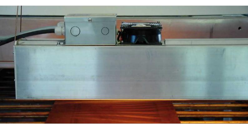
Simply Constructed Modules contain one or more infrared emitters. They can be easily retrofitted into existing production plants and because of their long operation lives, they are extremely cost-efficient.
