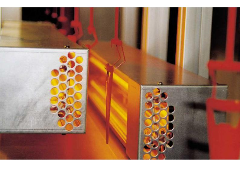
The MX module with its integrated control unit represents a system solution for the total heating process. Each module is optimised in size and wavelength to deliver energy effectively and efficiently at the surface to be heated.
