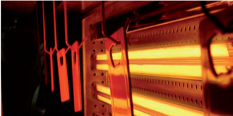
Carbon twin emitters flow and cure powder coatings efficiently
