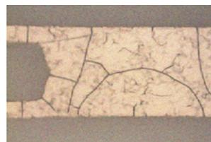
**Fig. 4: Cracks in layer applied by PVD**
