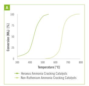
Ruthenium has been found to be the most active metal for the ammonia cracking reaction, strongly outperforming nonruthenium catalysts A.
