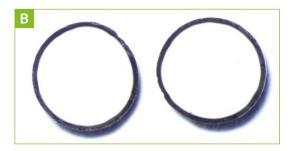
The remarkable performance of rutheniumbased catalyst systems may be attributed to two factors: i) A well-defined distribution of the active material, as is shown in <sup>B</sup> (Ruthenium is primarily located in the outer shell of the pellet), and ii) a narrow nanoparticle size distribution, as is evident in <sup>C</sup>.
