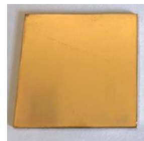
GG 991BD-H T on top of barrier solution RL A4841-H/2 BLUE H fired on 625 Inconel
