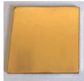
GG 991BD-H T on top of barrier solution RL A4841-H/2 BLUE T fired on 625 Inconel
