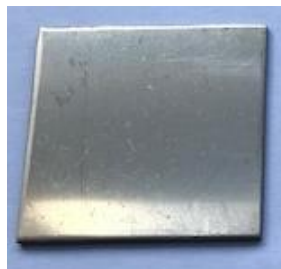
RL PT APP 100A-H BROWN T on top of barrier solution RL A4841-H/2 BLUE T fired on 625 Inconel
