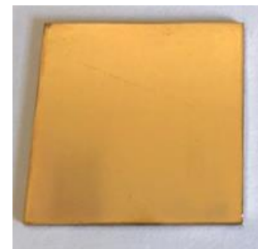
GG 991BD-H T on top of barrier solution RL A6294XB/2 BLUE T fired on 625 Inconel
