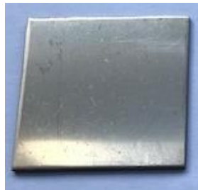
RL PT APP 100A-H BROWN T on top of barrier solution RL A6294XB/2 BLUE T fired on 625 Inconel
