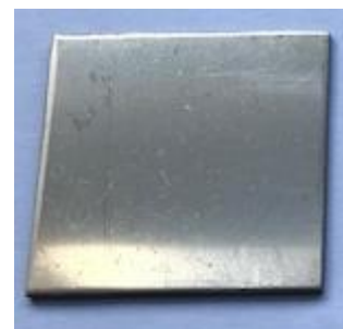
RL PT APP 100A-H BROWN H on top of barrier solution RL A4841-H/2 BLUE H fired on 625 Inconel
