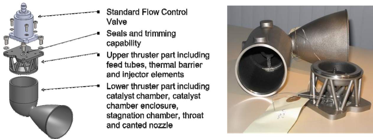
Figure 5. Final Thruster Design and printed Hardware
