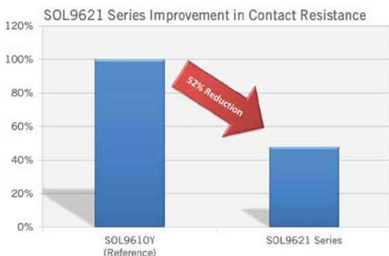
Figure 1. Heraeus' SOL9621 Series demonstrates a reduction in contact resistance (relative to SOL9610Y) on cells using standard emitter to ultra-low doped emitter wafers. Results are performed on 90–100 /sq. multicrystalline wafers. The SOL9621 Series demonstrates improved electrical performance.
