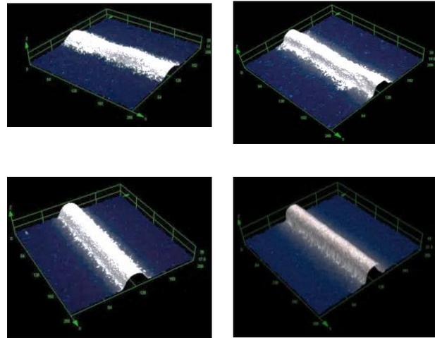
Fig. 10 Comparison of finger cross sections of the four applied technologies. Single and double screen printing are depicted in the top row, the two dispensed fingers with ordinary paste and rheologically adapted paste in the bottom row.
