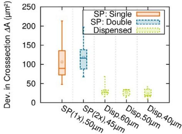
Fig. 7 Comprison of finger homogeneity of the applied technologies by means of the standard deviation in finger cross section area  $A_f$ .
