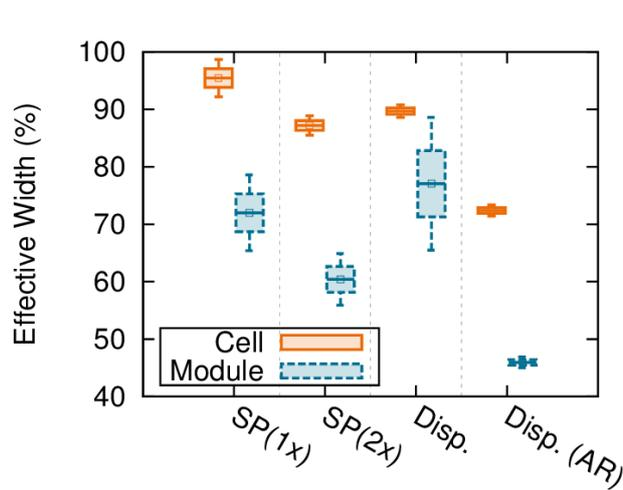
Fig. 9 Effective finger widths on cell and module level in comparison for different printing technologies.
