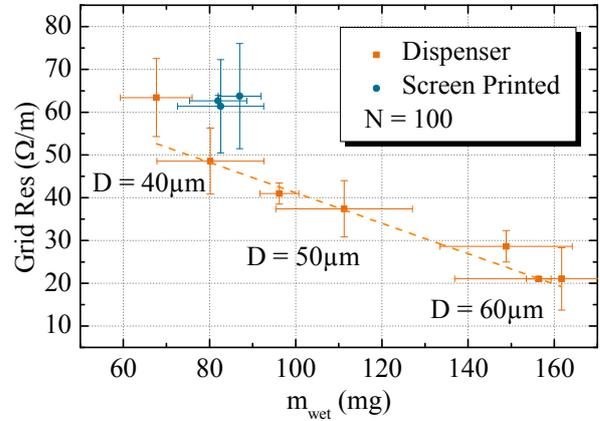
Fig. 8 Correlation of wet paste consumption and grid resistance  $R_{\text{Grid}}$  for dispensing and screen printed solar cells, respectively.
