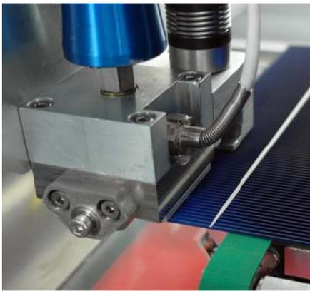
Fig. 3 Advanced version of the ten nozzle print head during cell manufacturing within the new dispensing platform.
