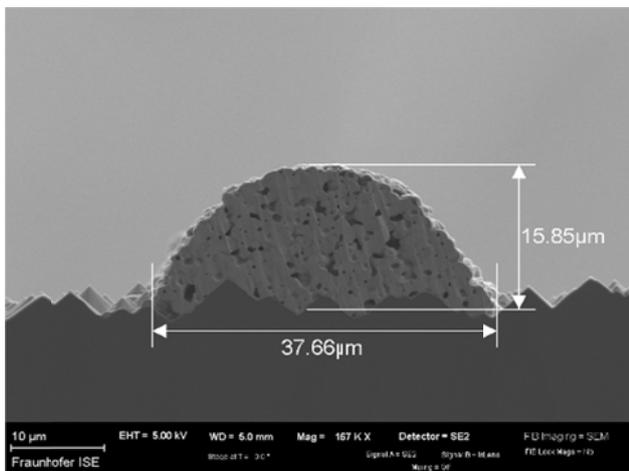
Fig. 1 Finger cross section of dispensed contact fingers using a new developed screen printing paste, printed in a parallel dispensing unit with a nozzle opening of just 40μm.
