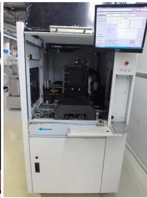
Fig. 4 Completely new developed, inline applicable dispensing platform at Fraunhofer ISE's PV-TEC.
