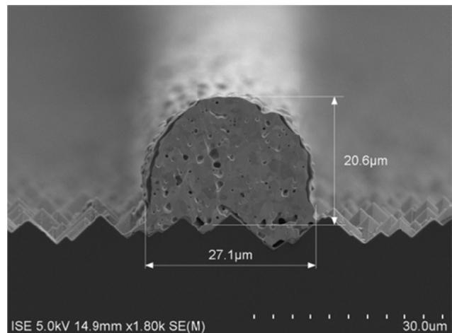
Fig. 2 SEM picture of finger cross section of dispensed contact fingers using a dispending paste with adapted rheology [10], printed in a parallel dispensing unit with a nozzle opening of just 40μm.
