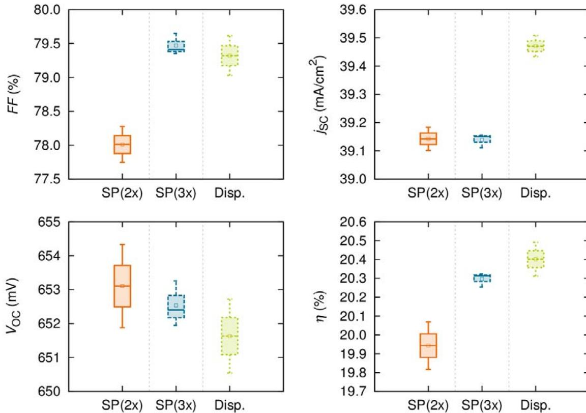
Fig. 12 IV-results of recent cell batch on industrial pre-processed and passivated Cz p-type material (PERC concept). All groups contain screen printed non-contacting busbars prior to the subsequent application of contact fingers by alternatively one or two additional screen printing steps or dispensing, respectively.
