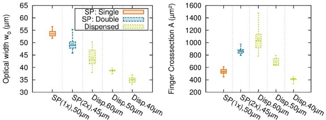
Fig. 6 Optical finger width (left)  $w_o$  and corresponding finger cross section (right) of different printing technologies with indicated screen opening width  $w_s$  and nozzle opening diameter  $D$ , respectively.
