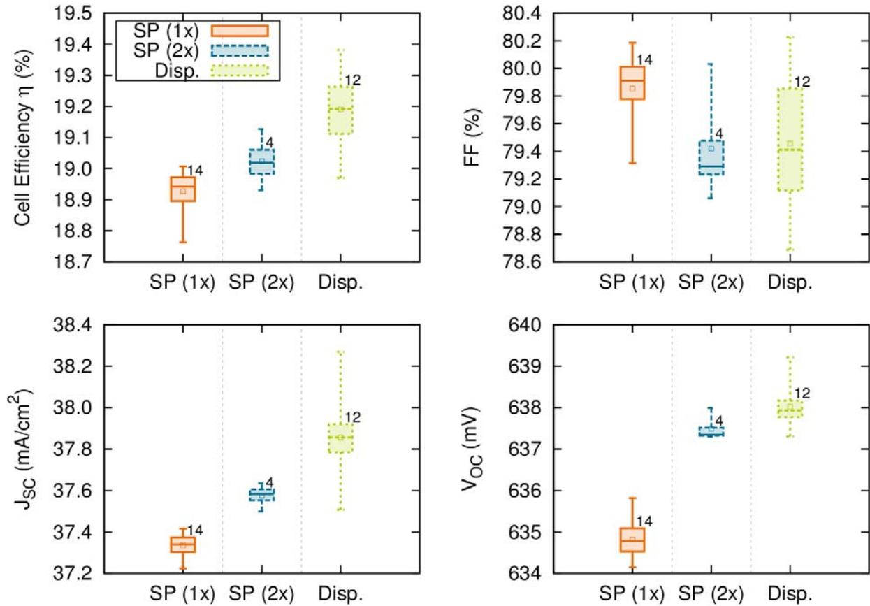
Fig. 11 IV-results of recent Al-BSF cell batch on industrial preprocessed Cz p-type material with an emitter sheet resistance of  $R_{sh}=90\Omega/sq$ .
