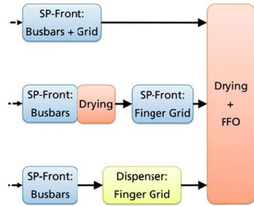
Fig. 5 Concepts for inline integration of different printing approaches. Standard single printing (top route) is compared with dual/double printing (second route) and dispensing (bottom route).
