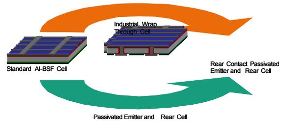
**Figure 1:** Fraunhofer ISE technology roadmap for future cell devices
