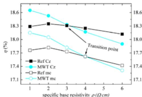
**Figure 5:** 2D “Sentaurus Device” simulation of a MWT and conventional solar cell [25]. The simulation shows a transition point depending on the bulk lifetime (mc, Cz) and base resistivity. Boron-oxygen induced degradation effects of the bulk lifetime are not regarded. The absolute values for the bulk lifetime are based on estimated input parameters, so especially for mc-Si an overestimation is probable.
