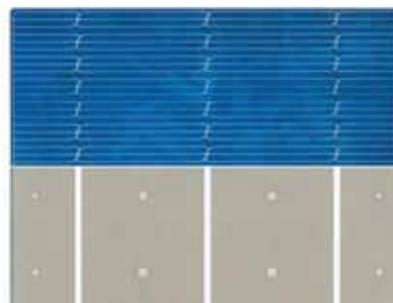
**Figure 4:** Picture of the front and rear of a typical mc-MWT solar cell (156x156 mm<sup>2</sup>) with three continuous rear busbars processed at Fraunhofer ISE [24].
