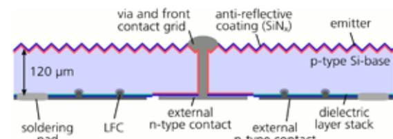
**Figure 2:** Schematic structure of the MWT-PERC devices presented in this work.
