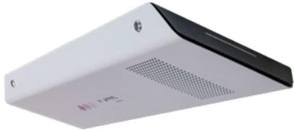
**Soluva® Air V** continuously purifies the cabin air in buses and other public transportation vehicles during the journey – reliably and efficiently. The UV light immediately destroys viruses and their mutations, bacteria and other pathogens. The UV-C air purification device simply mounts on the passenger cabin ceiling to provide increased protection for travelers. Its use is already proven in many public buses.
